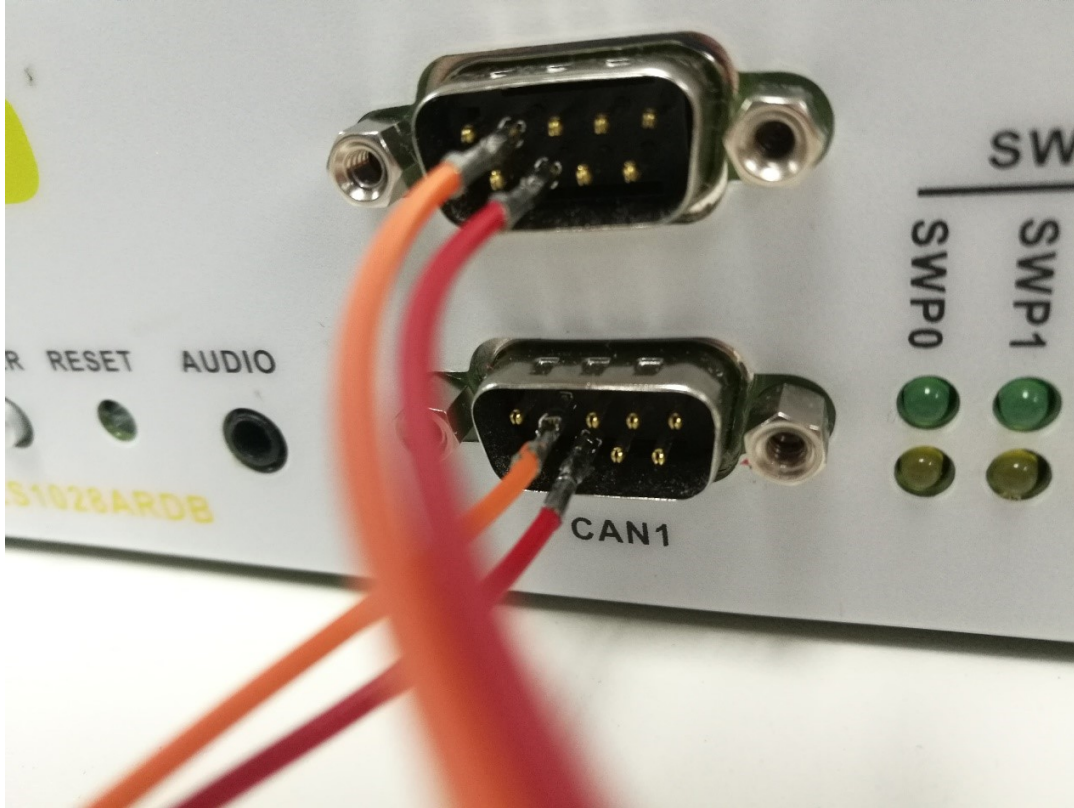
Figure 54. Physical connection for CAN using LS1028ARDB
