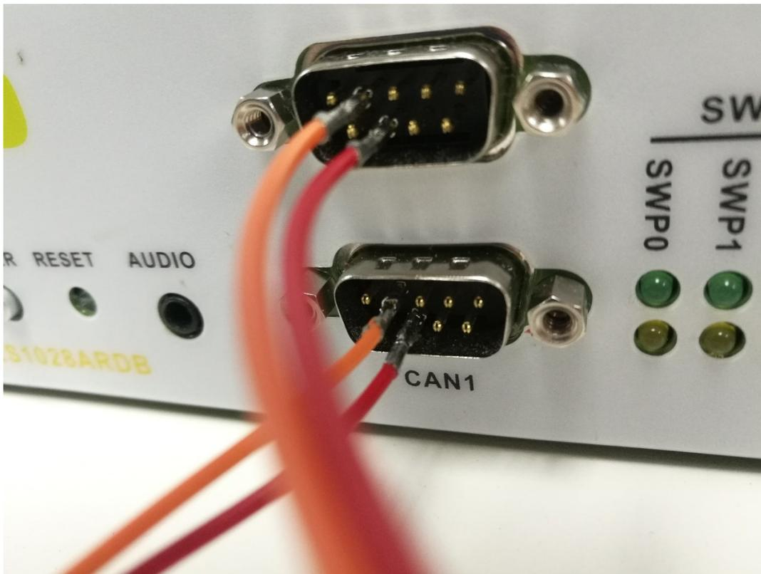
Figure 45. Physical connection for CAN using LS1028ARDB
