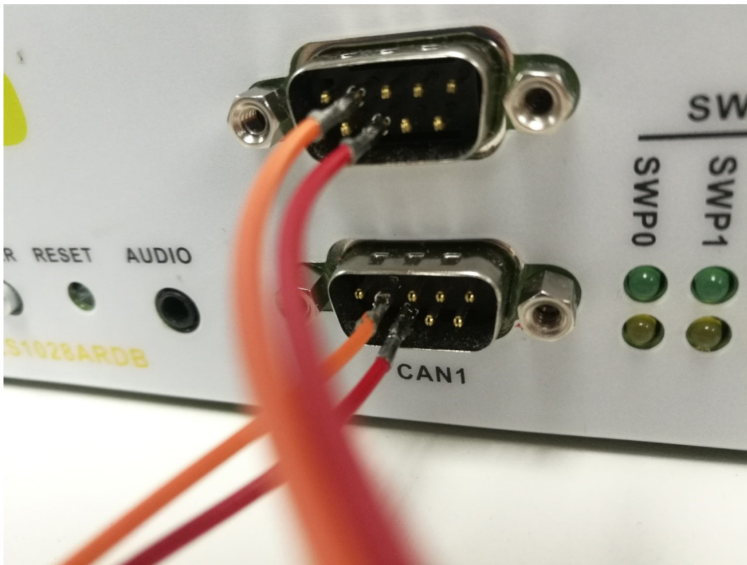
Figure 79. Physical connection for CAN using LS1028ARDB
