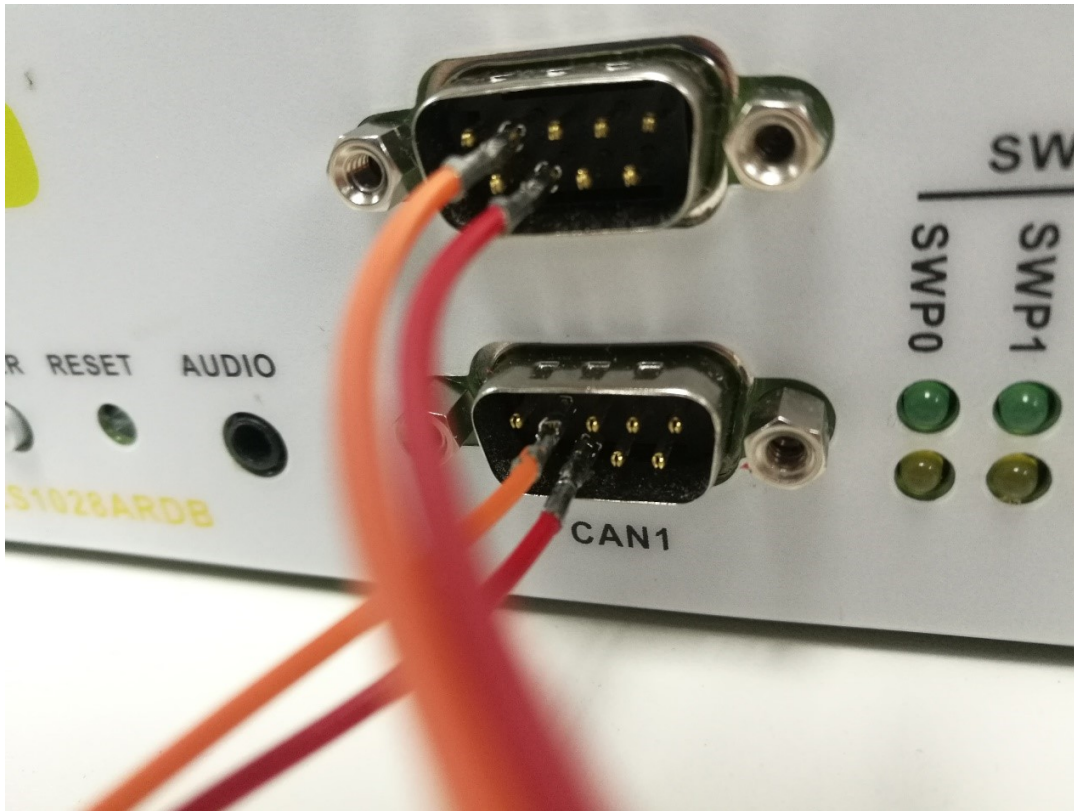
Figure 89. Physical connection for CAN using LS1028ARDB
